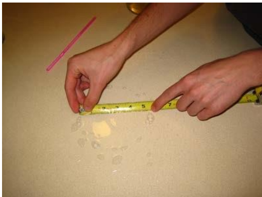
Picture 7. Measuring the bubble diameter.
